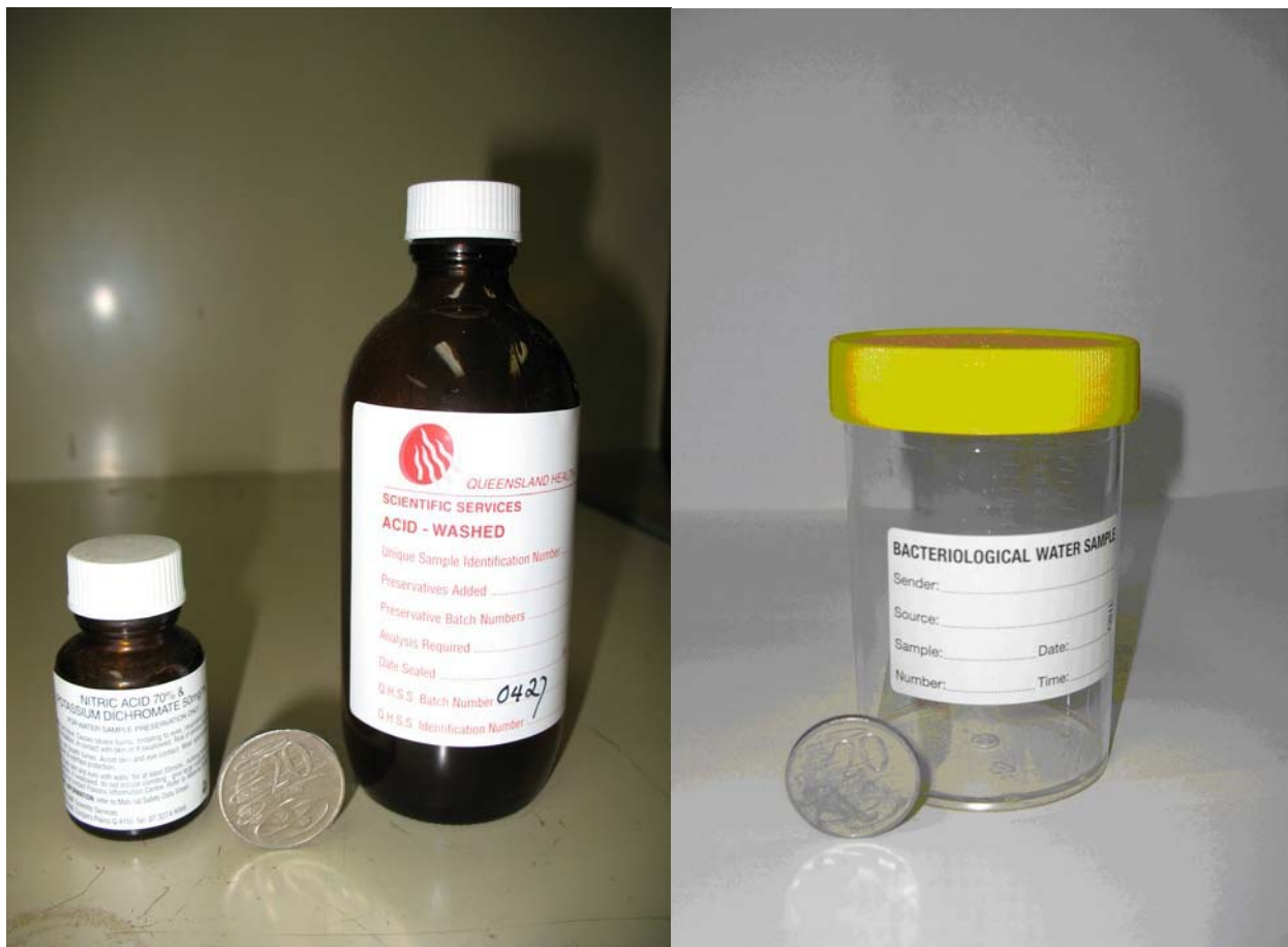
MB/G7 – Red label acid washed 250mL glass bottle for mercury; preservative consists of 2mL concentrated nitric acid plus 2mL potassium dichromate.
