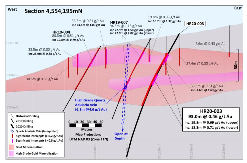
**Figure 5:** Cross section 4,554,195mN at Bells with drilling results highlighted from HR20-003. The drilling results are shown relative to the existing interpretation of the shallow gold mineralisation based on the historical drilling and the 2019 RC drilling (HR19-006 and HR19-007) completed by Rex at this location.
