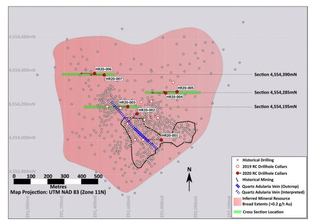
**Figure 2:** Plan view of the RC drill holes at Bells relative to the extensive historical drilling information and the broad boundary of the current Inferred Mineral Resource estimate.
