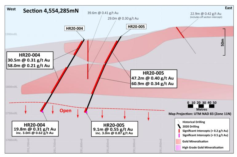
**Figure 4:** Cross section 4,554,285mN at Bells with drilling results highlighted from HR20-004 and HR20-005. The drilling results are shown relative to the existing interpretation of the shallow gold mineralisation based on the historical drilling information at this location.
