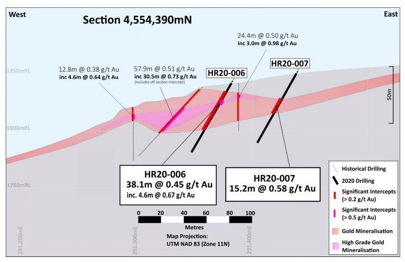
**Figure 3:** Cross section 4,554,390mN at Bells with drilling results highlighted from HR20-006 and HR20-007. The drilling results are shown relative to the existing interpretation of the shallow gold mineralisation based on the historical drilling information at this location (also reported earlier by Rex on 16 September 2020).
