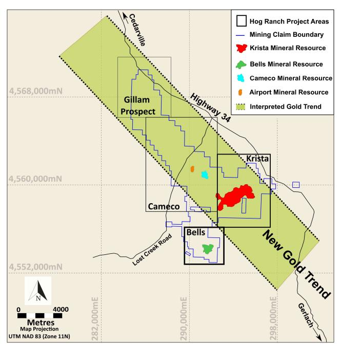
**Figure 1:** View of the updated mining claim boundaries at Hog Ranch, relative to the newly-defined Gold Trend which cuts through the host rocks at Hog Ranch and is interpreted to be the focus of significant gold mineralisation.
