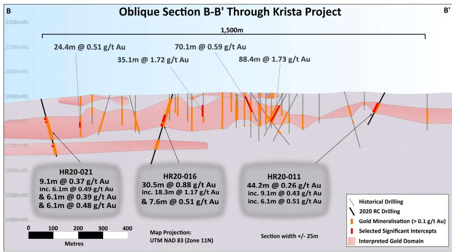
**Figure 4:** Oblique cross section B-B' (see Figure 3) with drilling results highlighted from HR20-011, HR20-016 and HR-021. The drilling results are shown relative to the existing interpretation of the shallow gold mineralisation based on the historical drilling information at this location.
