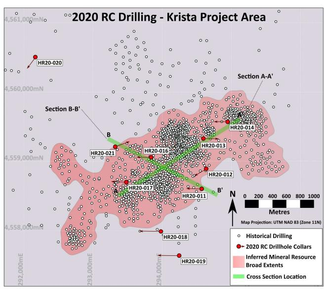
**Figure 2:** Plan view of the RC drill holes at Krista relative to the limits of the current Inferred Mineral Resource estimate. Drill holes that appear within these limits were designed to test for deeper extensions of gold mineralisation that are interpreted to exist outside of the currently defined Mineral Resource.
